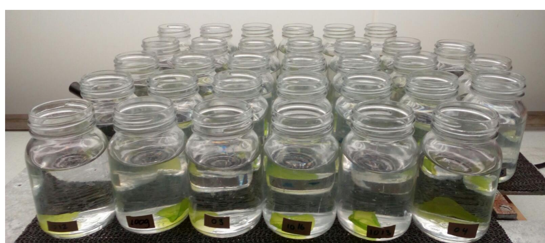
Figure 2. Experimental setup, punched out U. lactuca tissue in 200 ml medium on a rotating table (100 rpm) for mixing and gas exchange.
